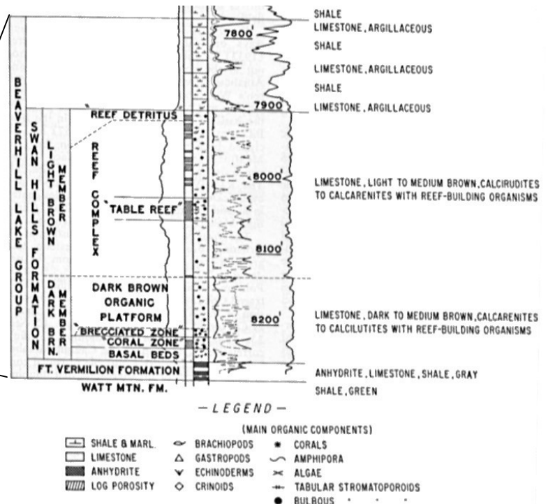
FIG. 8.—Typical Beaverhill Lake section in Swan Hills field, Alberta. Well is Home Regent Swan Hill 4-28-67-10-W5M. KB elev. = 3,322.1 ft. Well was cored almost completely through Swan Hills Formation permitting excellent control for facies divisions shown. Depths in feet below KB.
